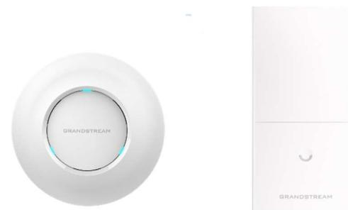
Designed for small to medium sized businesses, multiple floor offices, commercial locations and branch offices, the GWN7600 is a mid-tier 802.11ac Wave-2 WiFi access point. It supports up to 1.27Gbps, over 450 concurrent WiFi clients and up to a 165 meter coverage range. To ensure easy installation and management, the GWN7600 uses a controller-less distributed network management design in which the controller is embedded within the product's web user interface.
